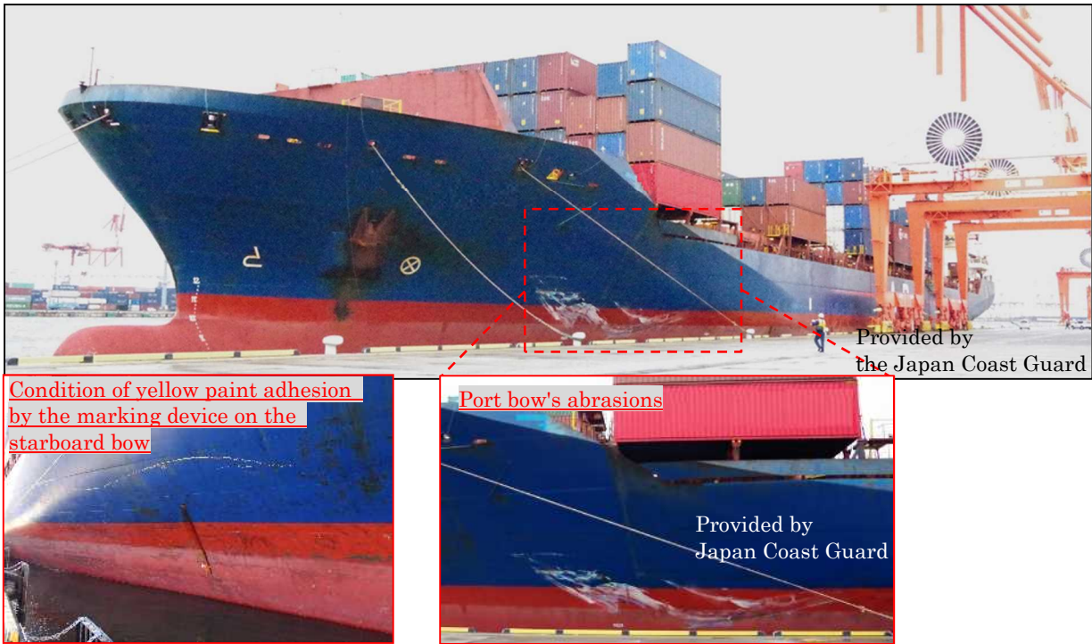
Photo 1 State of damage to Vessel A
